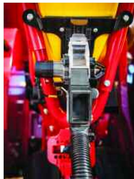
*Väderstad's Tempo electrically driven Gilstring Seed Meter delivers singulation and precision at high driving speeds.*
